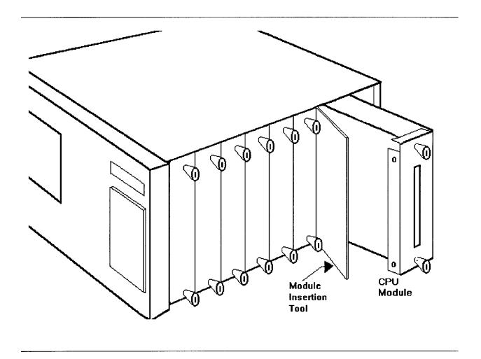
Figure 1 Position of Processor Module and Insertion Tool
